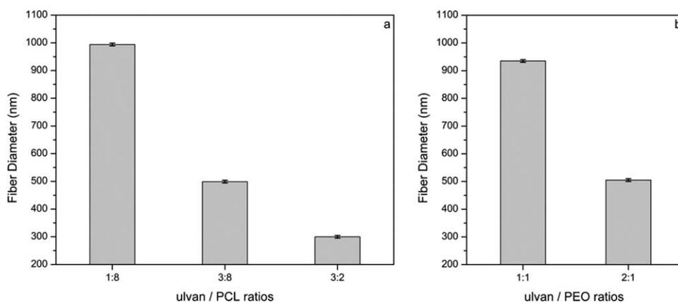
**Figure 4.** Average diameters with standard error bars of (a) ulvan/PCL and (b) ulvan/PEO nanofibers in relation to the polymer ratios.
