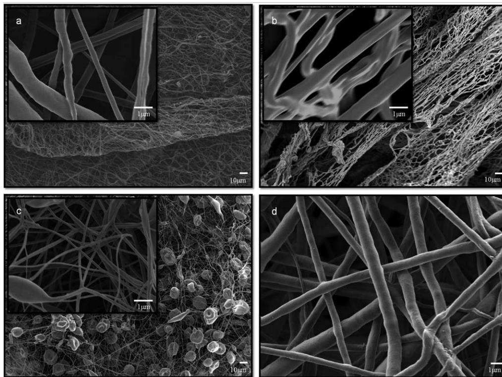
**Figure 1.** SEM images of fibers of ulvan/PCL at (a) 1 : 8, (b) 3 : 8, and (c) 3 : 2 ratios and (d) PCL.
