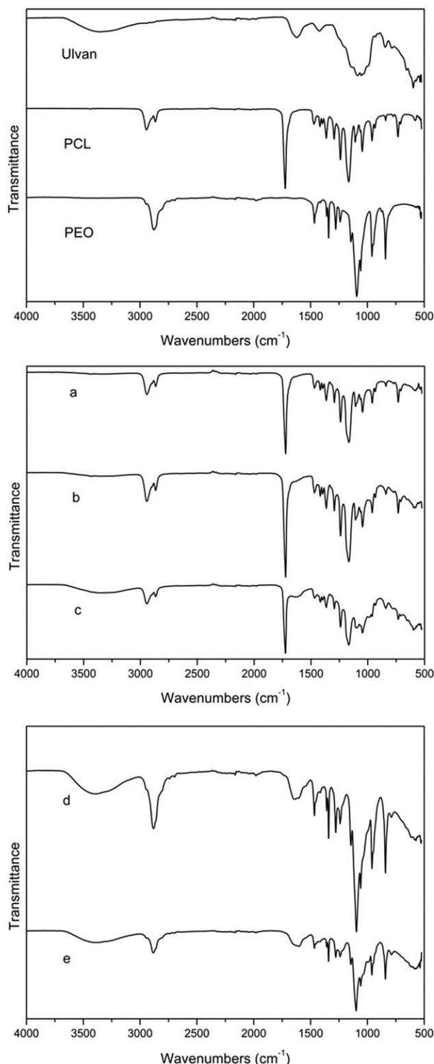
**Figure 3.** FT-IR spectra of (A) ulvan, PCL and PEO; (B) ulvan/PCL at (a) 1 : 8, (b) 3 : 8, and (c) 3 : 2 ratios; (C) ulvan/PEO at (d) 1 : 1 and (e) 2 : 1 ratios.
