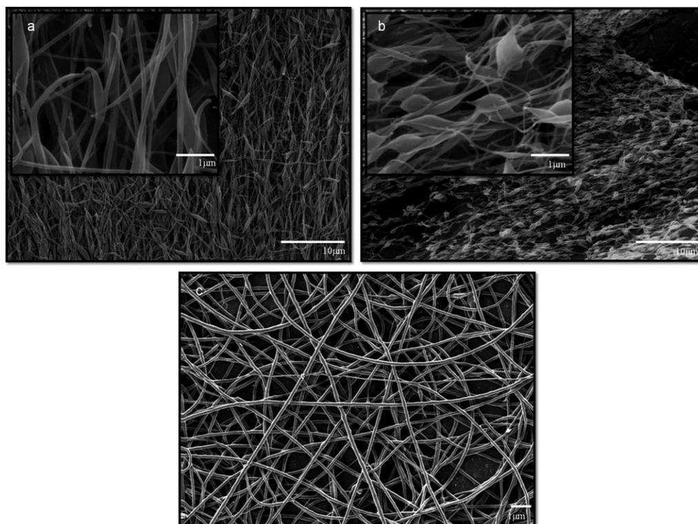
**Figure 2.** SEM images of fibers of ulvan/PEO at (a) 1 : 1, (b) 2 : 1 ratios, and (c) PEO.
